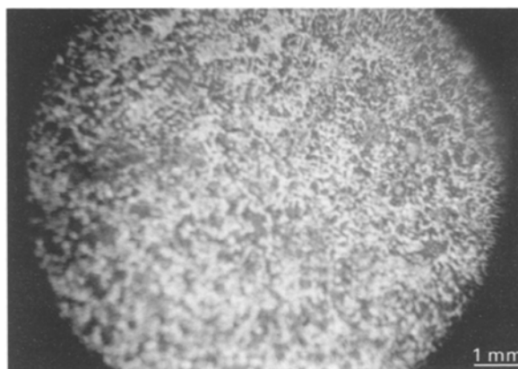
Figure 6 Reflected light micrograph of indium-tin alloy.
